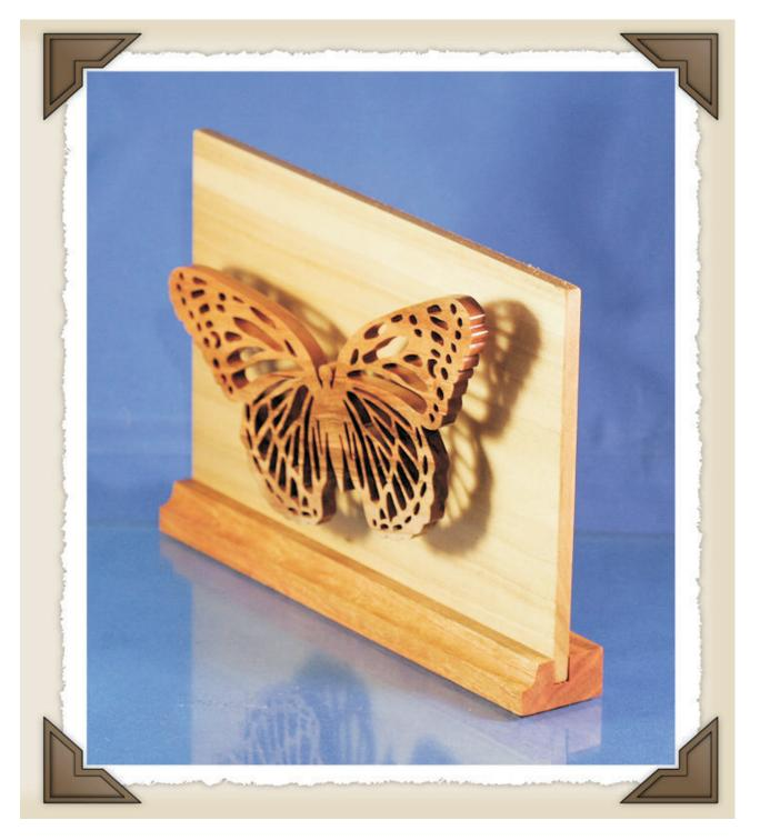
The base is constructed from 3/4" x 1  $\frac{1}{2}$ " x 8  $\frac{1}{2}$ " stock. Cut a 1/4" groove in the base to hold the backer board. Use a small block of wood behind the butterfly body to lift it  $\frac{1}{2}$ " off the back. 1/4" Thick
