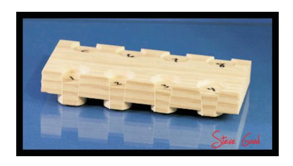
Use this gauge to make it easier to determine the correct starting angle of a scroll saw relief cut.
