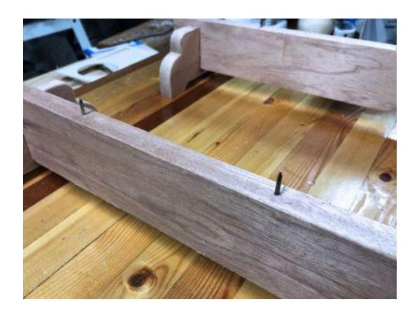
Pre-drill and insert cut off nails for holding piece off the top of the bench top saw horses. Great for painting and finishing.
