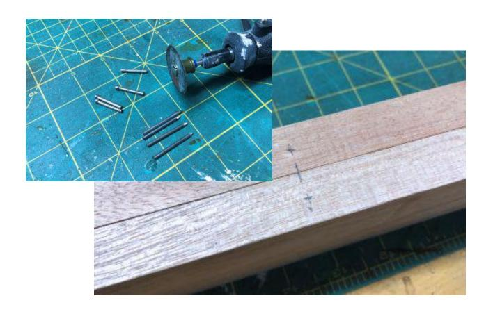
You can drill as many nail holes as you need. I put two on each horse. Leave about 1/2" of the nail sticking out.
