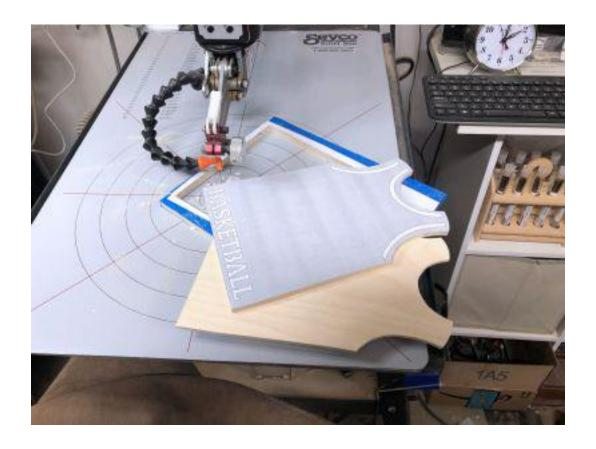
Stack cut the outside cuts of the jersey and the backer board. The remove the backer board and drill the interior holes for the interior cuts. Make the cuts.
