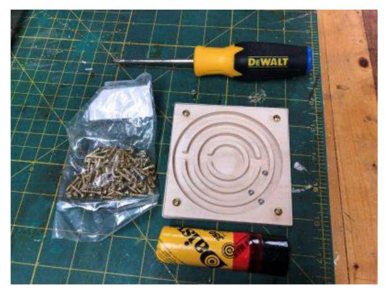
Pre-drill the holes to screw the acrylic to the top of the game. Install 3 Bb's and screw on the acrylic
