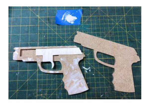
Carefully glue the pieces together so you don't glue the trigger in place. It needs to slide smoothly.
