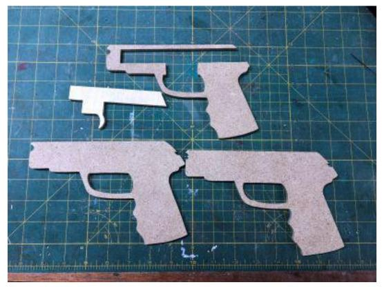
Here are the four parts. I used MDF for all the parts except the trigger. I used Baltic birch plywood for the trigger so it would have more strength.
