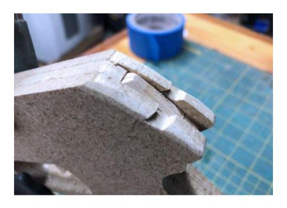
Notice how I slightly rounded over the rear of the gun. This allows the rubber band to release smoothly when the trigger is pulled.
