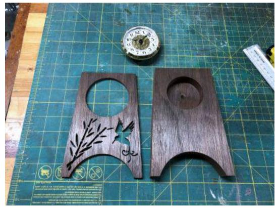
I used a 2 3/8" Forstner bit to cut the hole in the thick part of the clock. You can cut it with the scroll saw if you don't have the bit. Just cut slightly inside the pattern line and sand the hole for a snug fit of the clock insert.
