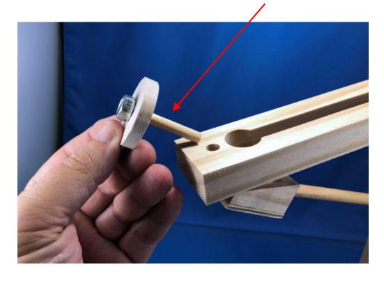
Drill pivot hole approximately 5 7/8 from the shovel end of the shaft. You want the shovel to hit the piston shaft dead center.
