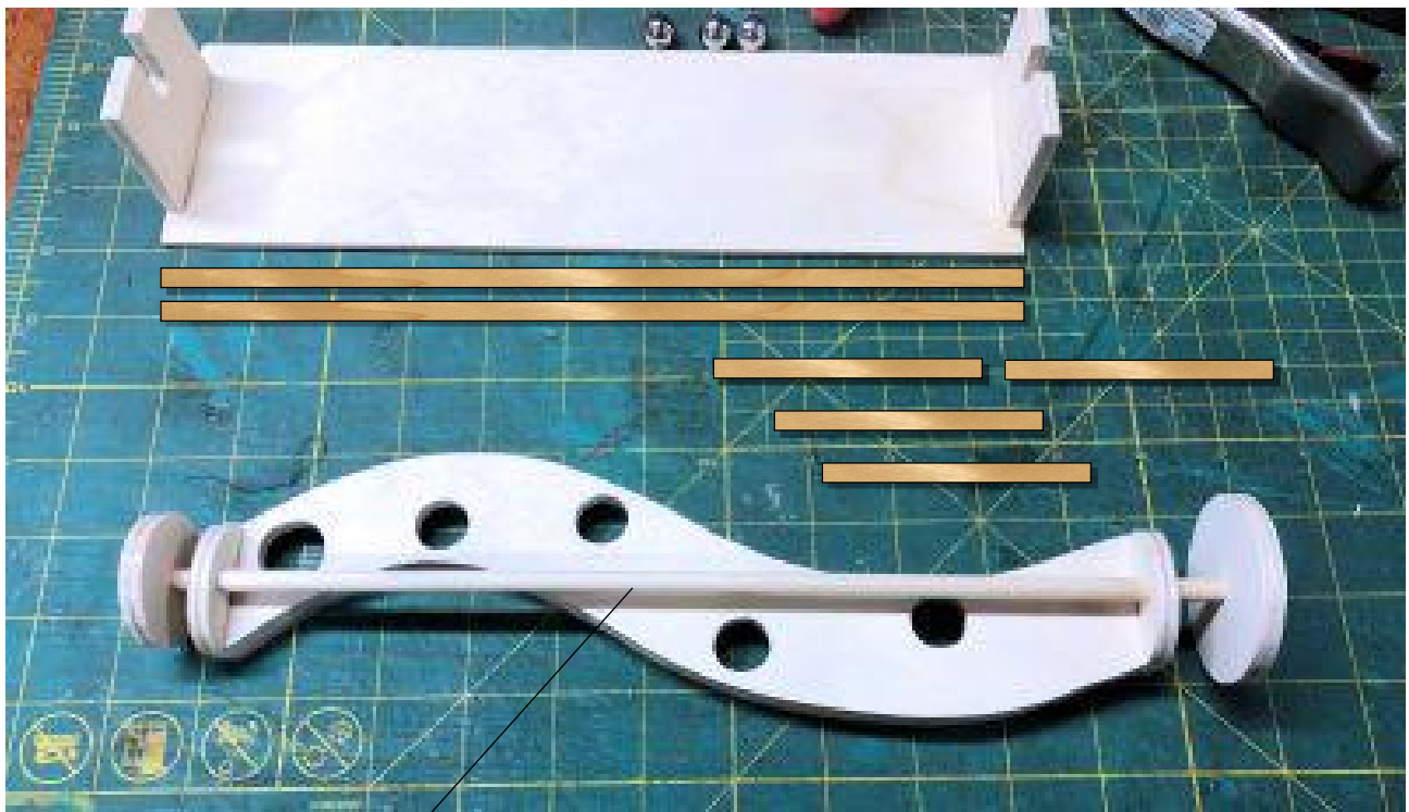
This dowel is 12" long and 1/4" diameter
