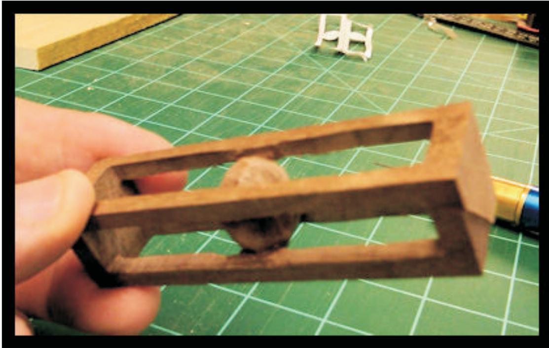
I'm just about to free the ball in this photo. Make very easy plunge cuts to free the ball. You have to be careful not to apply too much pressure to the cage as you round the ball.
