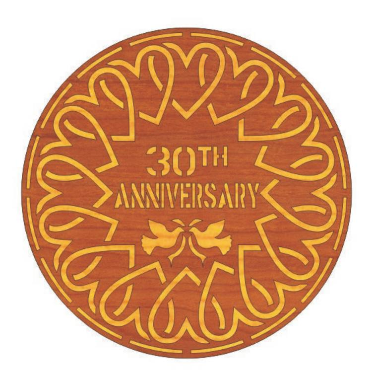
The plate can be cut as is or add a backer board for contrast. If you use a backer board stack the two plates then separate for the interior cuts. If you cut without a backer board use ½" thick wood. Use 1/4" for if you add a backer board.
