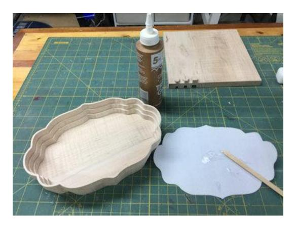
Telescope the plate out and apply glue sparingly. It's easy to get glue squeeze out that will mar the finish. Use a damp towel to immediately clean the extra glue off the exposes surfaces.
