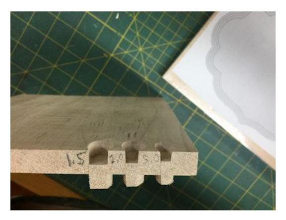
Make test cuts with the same material you will be cutting the project from. Tilt the scroll saw to a small angle and test to see how much projection you get before the piece wedges. In this case 1.5 degrees gave me what I needed.
