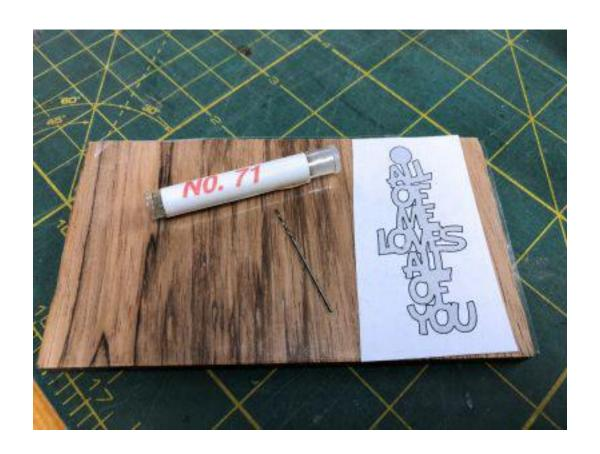
I used a #71 micro drill bit for all the interior holes.
