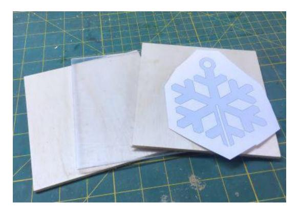
I am using 1/8" thick cast acrylic. The acrylic is much easier if you sandwich it between two pieces of Baltic birch plywood.
