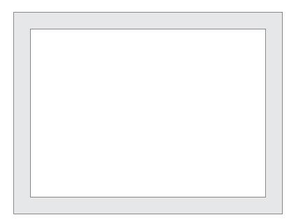
Inside wall will be glued to bottom. Cut from 3/4 inch wood or thicker.
