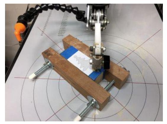
After you complete side one flip the piece in the blank and cut side two.
