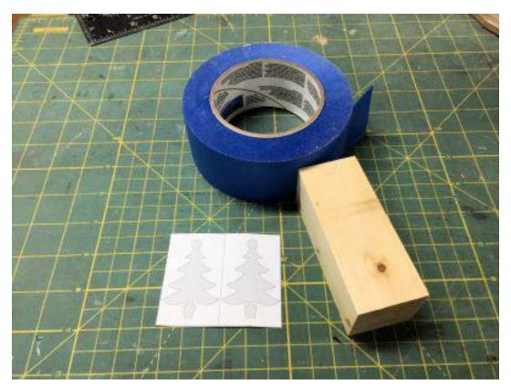
I used a standard construction grade 2X4 cut down to a 1.5" X 1.5" blank approximately 3.5" long.
