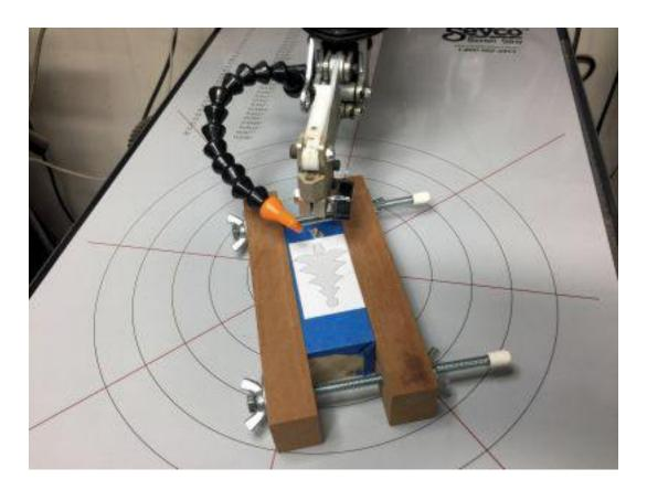
Drill an entry hole on through the blanks for the blade.
