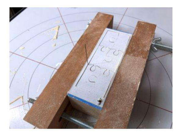
Cut side one then flip the piece to prepare to cut side two.
