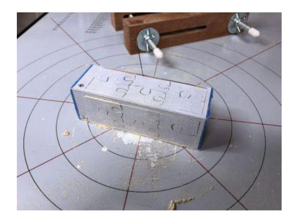
Remove the block from the jig and carefully dissamble the waste pieces from the block
