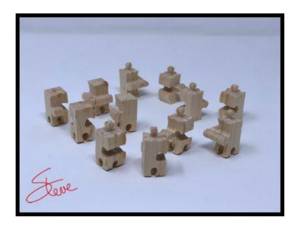
This puzzle needs accurate 90 degree cuts or it will not slide apart easily. Use a sharp blade and let the blade do the cutting. Don't force the cut or you will end up will bowed or slanted cuts.
