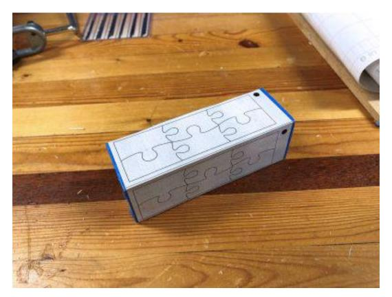
Wrap the pattern around a 1.5" X 1.5" X 4.25" Block covered with blue painters tape.
