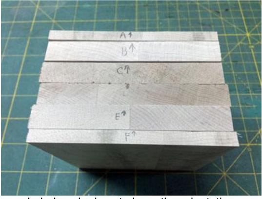
Label each piece to keep the orientation after you remove the pattern.
