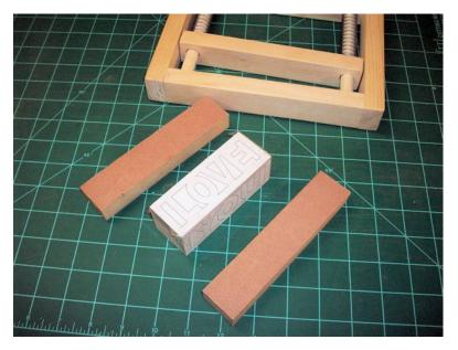
Wrap the pattern around two sides of the blank.
