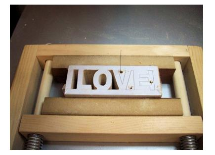
To cut this pattern it's best to have a clamp to hold the blank while you cut. Drill your interior holes. Cut the first side.
