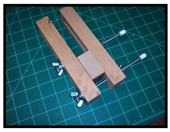
One of the bolts can be slid along the groove to adjust to the size of the project.
