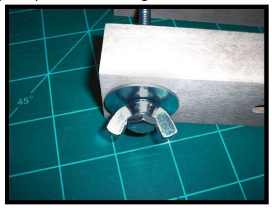
The hex head is captured by the wings of the wingnut and wont turn as to tighten the clamp.
