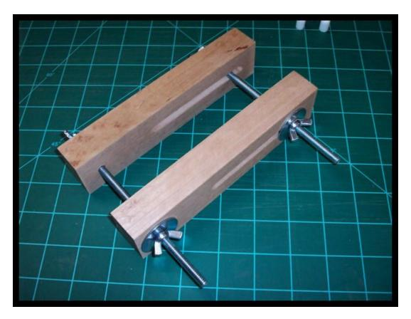
Install the two 1/4" wingnuts on the bolts.
