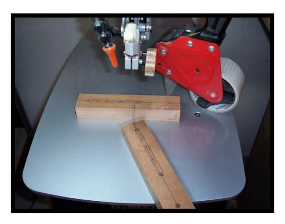
Cut the slot in both blanks
