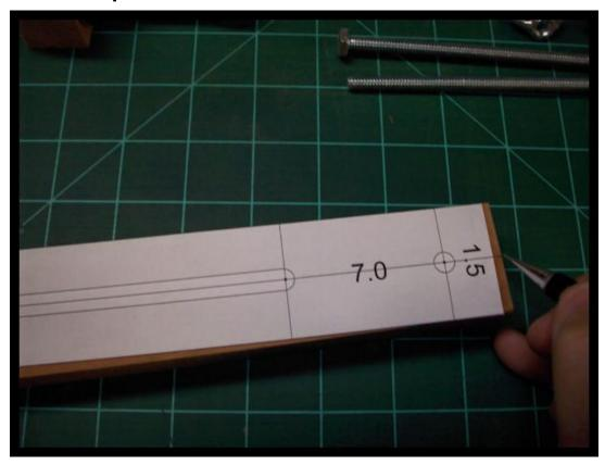
Use the story stick to mark the center line and the location to drill the holes.
