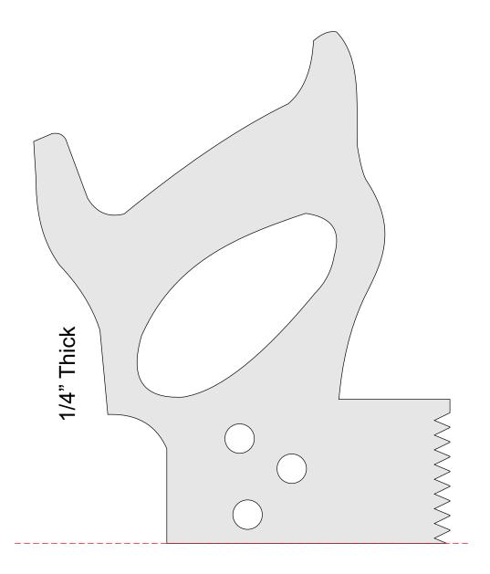
Fill holes with 1/4" diameter wooden dowel rod.
