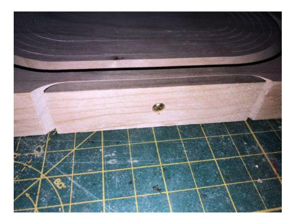
Pre-dril and countersink a hole to the base screw.
