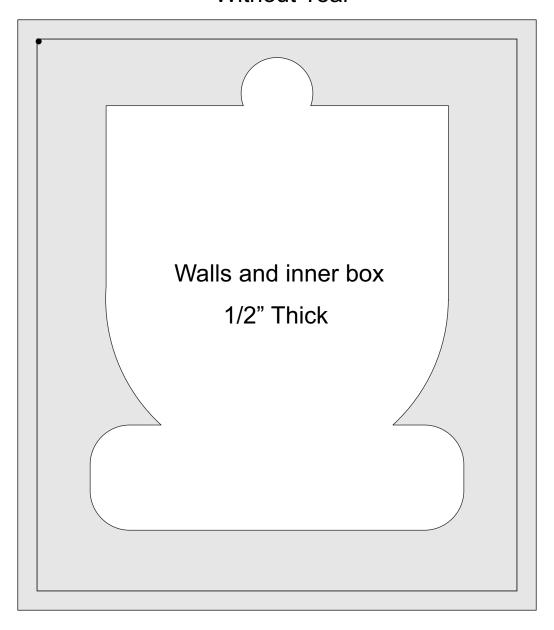
The outside walls and the inner section are cut from one piece of wood. The inner section can then be sanded for the best fit.
