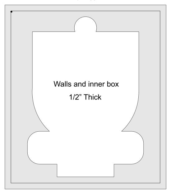
The outside walls and the inner section are cut from one piece of wood. The inner section can then be sanded for the best fit.
